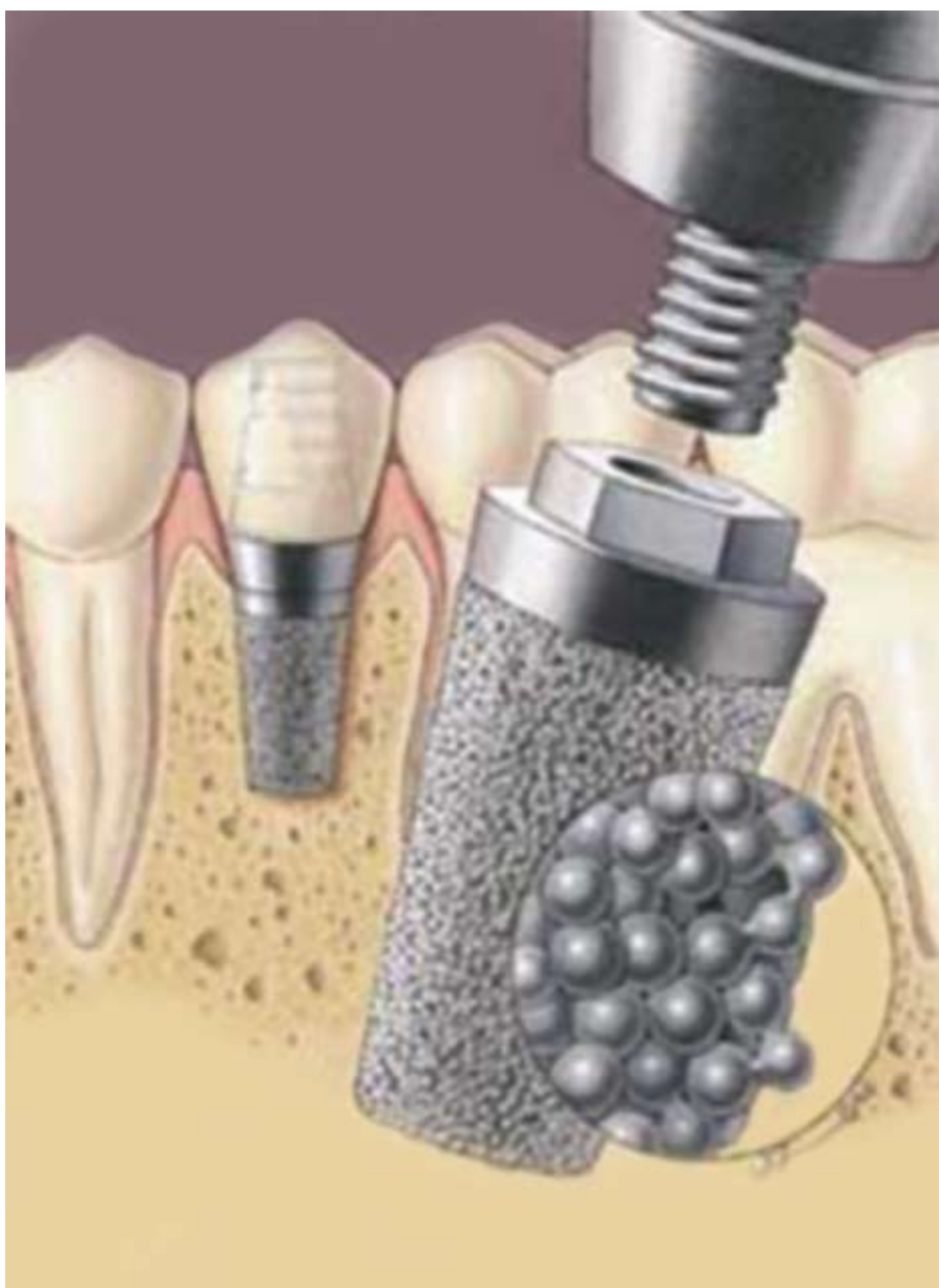
● Endopore Implant showing the unique three dimensional bone interlock.
